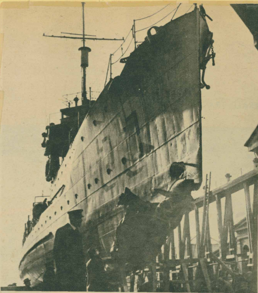
The Navy destroyer Paulding damaged its bow in ramming and sinking the submarine S-4 near Provincetown on Dec. 17, 1927. Forty Submariners died.
